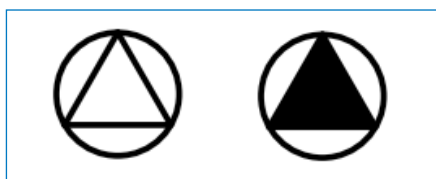
Figur 3.10 Pumpstation/tryckstegring respektive LTA-pump
