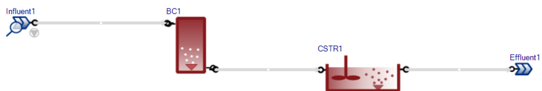
Figure 4 – Schematic overview of the virtual O 3 plant.
