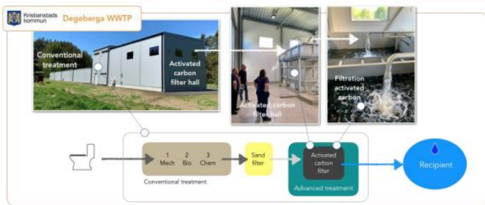
Figure 3. Overview of the full-scale advanced treatment with a combined Sand-GAC-filter at Degeberga WWTP in the summer of 2020.
